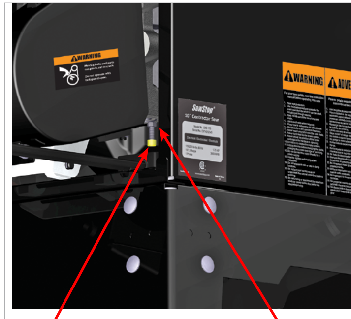
Lower elevation limit stop
