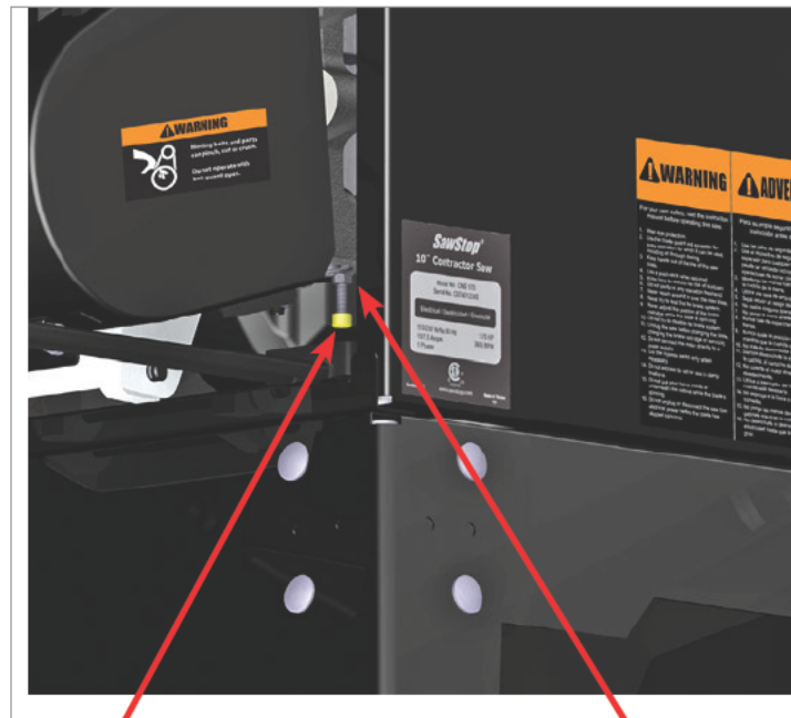
Lower elevation limit stop
