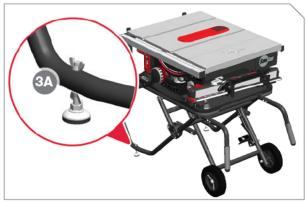
Make sure cart does not wobble. If needed, loosen wing nuts and adjust leveling feet, then re-tighten wing nuts (3A).
