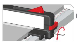
Once fence alignment is done, lock and unlock fence to make sure it is still tightly secured to rail. If fence slides while locked, or feels loose, use a 3 mm hex key wrench to tighten screw on front of fence.
