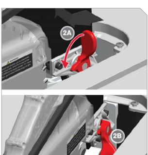
Rotate clamp handle down (2A, 2B) to secure blade guard in place. Install table insert.
