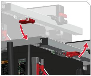
Extend table for rip cuts wider than 12" (30 cm). Flip handle out to unlock the table.
