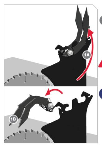
Leave pawls down to reduce likelihood of kickback. If you need to remove pawls, first remove guard, and then pull pawls back, up (1A) and forward to remove (1B). Store pawls in storage drawer (see page 23). To install pawls, reverse process.
