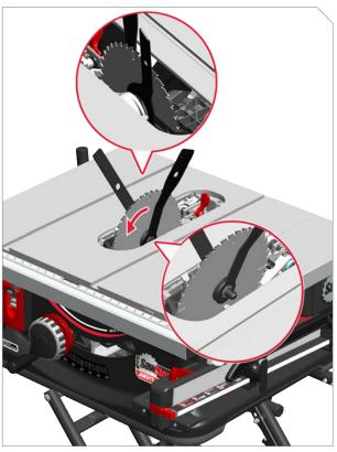
Loosen blade nut with wrenches. Remove nut and washer, change blade, and then reinstall washer and nut. Tighten nut with wrenchesdo not over-tighten. Make sure direction of blade rotation matches direction of teeth, as indicated by red arrow. Reinstall table insert and riving knife/blade guard.
