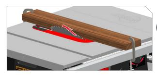
Start motor and slowly raise blade to highest elevation. This will widen slot for beveled cuts up to 45 degrees.
