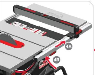
Slide the table to the right (4A) to extend. Flip handle towards the saw (4B) to lock table in place. The rails for the table must be fully extended to lock the handle.
