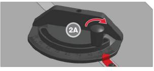
To adjust miter gauge angle, turn lock knob counter-clockwise, and then pivot miter gauge head until red pointer is above desired angle (+/- 60°). Tighten lock knob by turning it clockwise (2A) before making cut.
