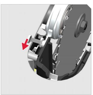
Loosen arbor nut and slide blade over slightly.
