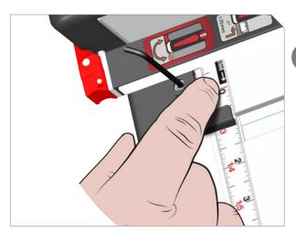
Slide lens by hand to correct location. If easier, you can also remove the fence and slide the lens from the underside of the fence.
