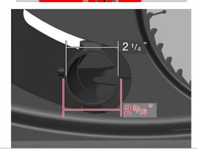
Connect suitable dust collector, which provides at least 170 CFM (4800 LPM) of airflow, to rear dust ports on saw and blade guard, using flexible connectors.
