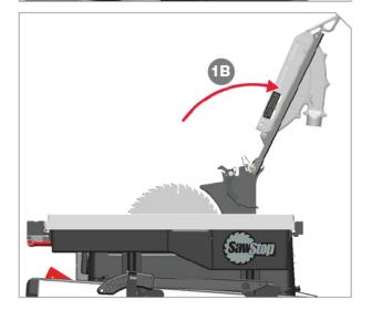
To provide easy access when changing blades, raise blade guard away from table. Pull guard forward (1A) then rotate it up and back (1B). Reverse steps to place the guard back in locked position for use.
