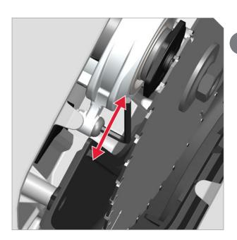
Use 4 mm hex key wrench to rotate bolt: if there was a gap, turn counterclockwise to move blade right until the gap is removed or less than 0.01" and clockwise to move blade left.
