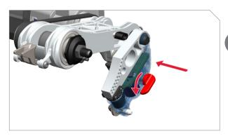
Slide new brake onto both pins. Insert key and rotate 1/4 turn counter-clockwise to lock in place. Reinstall riving knife/blade guard and table insert.
