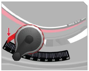
Blade tilt angle is indicated by position of red pointer over tilt scale.
