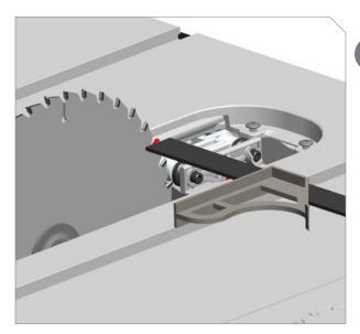
Set combination square parallel with right miter slot. Extend ruler until it lightly touches the side of the marked tooth. Tighten the locking knob on the combination square.
