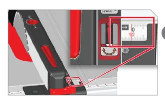
Raise blade fully. Make sure the table is fully retracted. Move fence so its left side rests against right side of blade. If indicator lens reads 0" (0 mm) on ruler, no adjustment is needed. If indicator does not read 0" (0 mm) proceed to next step.
