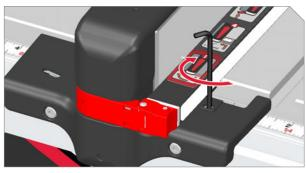
Tighten bolt. Check position of lens and make further adjustment as necessary.
