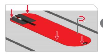
Install new table insert. Adjust leveling screws until table insert is level and slightly below table (see page 54).
