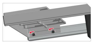
Use a 4 mm hex key wrench to SLIGHTLY loosen the two screws between front rail and extension table. Push down or pull up on extension table as necessary to correct alignment.
