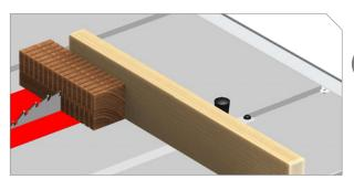
As needed, flip workpiece over and make another series of cuts, offset from first set, using same method.
