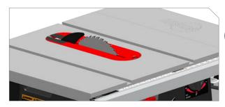
Stop motor and turn saw off. Remove wood and clamps. Remove table insert and install riving knife or blade guard (see page 30). Reinstall insert.
