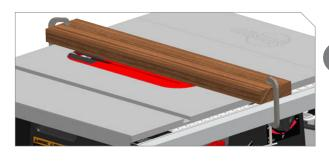
Lower blade to lowest elevation and turn off motor.
