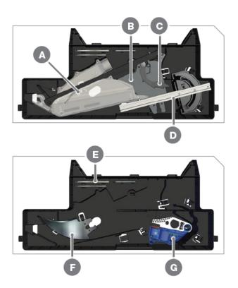
The drawer stores items in two layers, with the riving knife and optional spare brake underneath.
