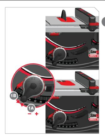
Rotate elevation hand wheel clockwise (1A) to raise blade, or counter-clockwise (1B) to lower blade. A single rotation adjusts blade elevation from fully lowered to fully raised, and vice versa.
