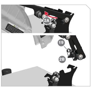
To completely remove the blade guard, rotate up and pull forward (2A) until the guide and height adjustment wheels are clear of the brackets (2B). Continue to lift and rotate until the top guard spring (19) releases from the bracket.
