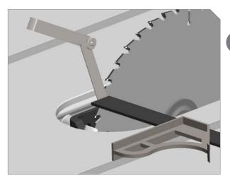
Now rotate the blade so the marked tooth is at the front of the blade. Move the combination square to align with the tooth. If there is a gap, measure the gap with a feeler gauge. If measurement is within 0.01" (0.025 mm), no adjustment is needed. If not, proceed to next step.
