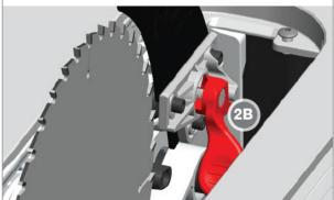
Rotate clamp handle down (2A, 2B) to secure riving knife in place. Install table insert. Reverse steps to remove riving knife.
