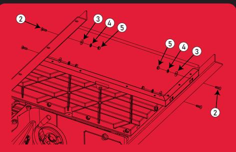
• The extension table mounts to the rails with bolts that pass through holes in the rails and extension table. Take four M8x1.25x25 flat head socket bolts (2) and insert one bolt into each of the remaining holes in
