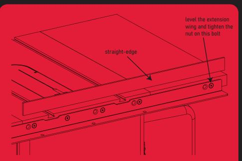
Use a straight-edge to level the rear edge of the left extension wing to the cast iron table top. You may have to pull up or push down on the outer edge of the extension wing to level it. Once the rear edge of the left extension wing is level, use a 5 mm hex key and a 13 mm wrench to
