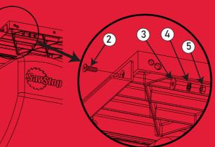
Take two M8x1.25x25 flat head socket bolts(2) and insert one through the open hole at the end of each extension wing.
