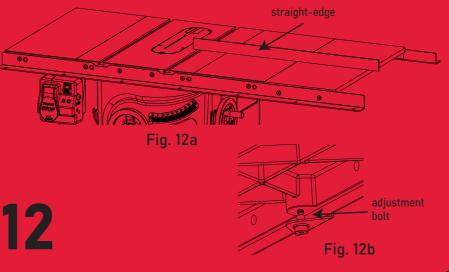
• The holes in the bottom of the front rail are oversized to allow you to adjust the position of the main tube on the rail. To set the main tube in
