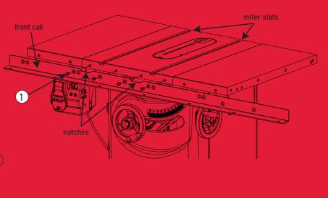
• Use a straight-edge to level the front edge of the left extension wing to the cast iron table top. You may have to pull up or push down on the outer edge of the extension wing to level it. Once the front edge of the left extension wing is level, use a 5 mm hex key and a 13 mm wrench to fully tighten the nut on the bolt that mounts the left extension wing to the front rail. Repeat this process to level the front edge of the right extension wing.
