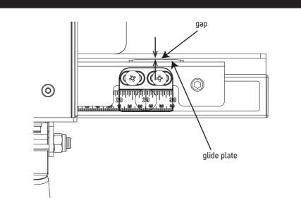
• Next, move the fence to the right end of the main tube, repeat the process described in step 17 to position the main tube, and tighten the right-most bolt. Once both ends of the main tube are adjusted correctly, use a 13 mm wrench to tighten the remaining M8x1.0x16 hex head bolts to mount the main tube to the front rail. Be careful not to overtighten
