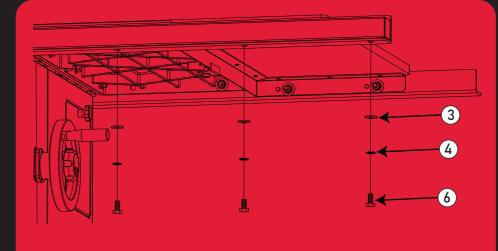
Locate the main tube and remove seven M8x1.0x16 hex head bolts, seven M8x23x2 washers, and seven M8 lock washers from the fence assembly hardware pack. Position the main tube on the horizontal portion of the front rail with the rulers facing up and the 12 inch ruler on the left. The powder coated surfaces of the main tube and rail can be slick, so be careful that the main tube does not fall off the rail. Align the noles in the rail with the holes in the bottom of the main tube. Place an
