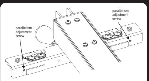
Press down on the fence handle to clamp the fence to the main tube. If the fence does not clamp tightly enough to hold its position against a moderate amount of force, you can increase the clamping pressure by turning both parallelism adjustment screws clockwise using a 3 mm hex key. Those screws are located in the vertical portion of the fence cross-bracket. Alternatively, if too much force is required to push the
