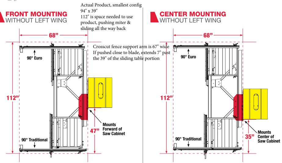
When the crosscut fence material support arm is fully extended, it adds an additional 35" to the width of the footprint and 37" to the length.
