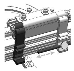
Alternatively, you can re-position the long steel rod in either of the flip stop arms (slide it left or right) and secure it in place by just one of the thumb screws (as shown above). The tip of the rod then becomes the stop for your workpiece.
