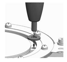
3. If your machine is equipped with a "T" shaped miter slot, install the T guide at the tip of the miter bar using a 5mm hex wrench.
