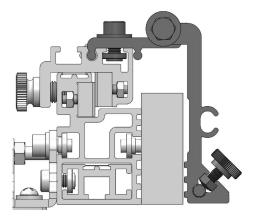
Reassembly is now complete. The above image shows the flip stop in the forward slot of the carrier to provide the necessary clearance for the sacrificial fence (also shown).
