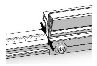
The measuring tape is held into the extension extrusion by friction and is not glued. By design, it does not move freely, but with some effort, it can be adjusted as described.
