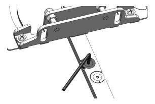
When the miter bar fit is too tight, consider removing the black, fixed guide-discs from the miter bar.
