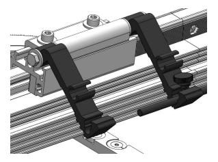
This ability enables you to establish stops for multiple cut lengths with setting the position of the stop carriage just once. Follow the steps below for setting cut length positions for each, individual flip stop.
