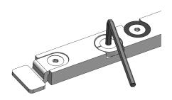
To access the rear adjustment disc, perform the following steps.
