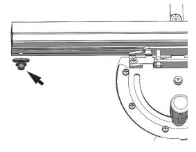
4. Insert the extension (A) into the opposite end of the main fence extrusion (B). Take care to align the rectangular nut (C) you re-located in the previous step with the T track of the extension as it is being inserted.
