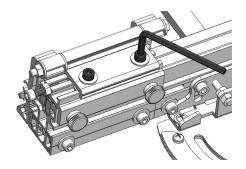
3. Loosen the nylon nut for the fine adjustment bolt shown. (No tools required.)
