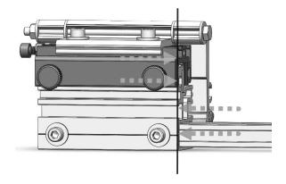
Next, secure the flip stop carrier with the thumbscrews you loosened in the previous step. Do not over tighten.
