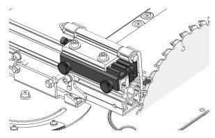
Set the gap (A) between the edge of the fence (B) and the saw blade (C) approximately 3/8" (9.5mm) from the blade. (See Setting Safe Fence Distance from Blade on page 9 for instructions.)
