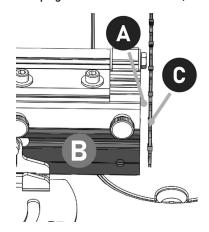
4. Loosen the socket head bolts indicated in the illustration below so that the flip arm assembly is freely moveable. Slide the flip arm so that the edge of the stop barely brushes the sides of the saw blade teeth. Take care to not deflect the blade.
