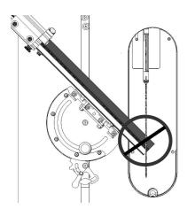
2. Adjust the fence to the left or right as needed to ensure an adequate margin of safe distance between the fence and blade is achieved.
