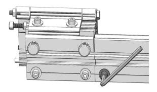
2. Pull the fence extension out and completely free of the main fence extrusion.
