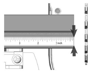
Loosen the nylon thumb screws on the back of the flip stop carrier and position the edge of the carrier to be also at the zero mark of the fence ruler.
