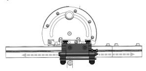
Secure the selected position of the dual flip stop assembly by re-tightening the nylon thumbscrews on the back of the dual flip stop assembly.
