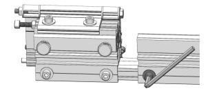
3. Re-secure the fence extension retention bolt using the supplied 5mm hex wrench to fix the extension at the selected position.
