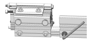
2. Loosen both nylon thumbscrews on the back of dual flip stop assembly at least one full revolution. Push the flip stop carriage forward slightly before moving it from its current location along the top of the fence.
