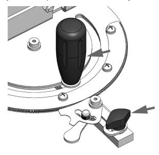
Remove your Scale Miter Gauge from the miter slot of your saw and remove guide disc from the miter bar as shown.
