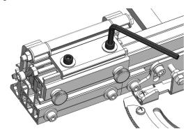
2. Slide the flip stop out of the rear T-slot of the carrier and move it to the forward slot.
