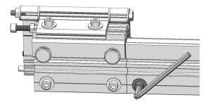
2. The telescoping fence extension now slides freely. Pull the fence extension to the desired length.
