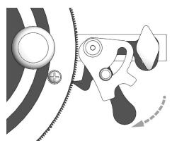
4. Tighten the *Grip* and the *Actuator Locking Knob*.
