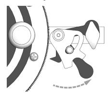
Loosen the Pivot Cursor Locking Knob (A) by turning it counter-clockwise. The vernier scale from which the miter angle is read (Pivot Cursor) can be pivoted forward again to rest against the protractor.
