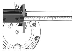
When using the flip stop in conjunction with the fence extension (measurements over 14 1/4" (362mm)), read the measurement from the lower ruler where the extension bar meets the extrusion of the main fence as shown in step 7.
