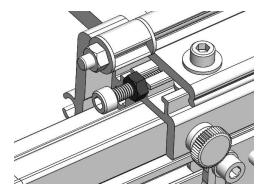
4. By turning the fine adjustment bolt (highlighted in the illustration below) you can shift the position of the dual flip stop to the left (counter-clockwise) or the right (clockwise).
