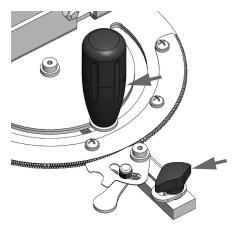
2. Pull the Pivot Actuator toward you to release its tooth from the mating detent on the Protractor.
