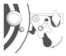
5. Re-tighten the Grip and the Actuator Locking Knob by turning them in a clockwise direction to secure your selected miter angle.
