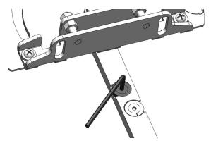
6. Using a precision reference square, align the fence against the *Miter Bar* and the fence head.
